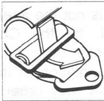
STEP 4: Fold back strap again and insert through bottom portion of buckle
